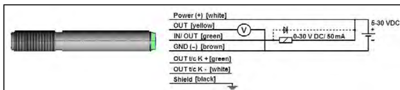
Figure 22: Open collector output as additional alarm output
