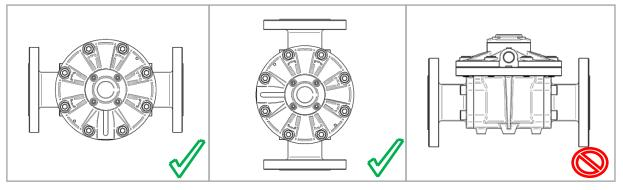
Liquid can flow in a horizontal direction, or a vertical direction, but in each case the rotor shafts must be in a horizontal plane. This is achieved by mounting the meter so that the terminal cover, or integral instrument display, is facing in a horizontal direction. For pulse output flowmeters the direction of flow is not important, as the output is non-directional.
