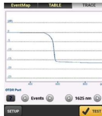
Splitter as seen on an OTDR trace
