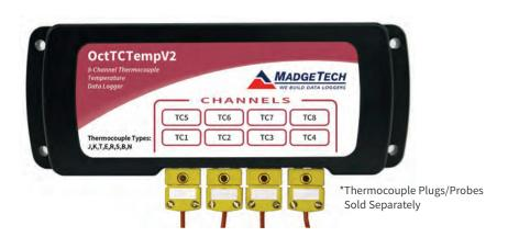
The OctTCTempV2 is an 8-channel thermocouple data logger with a reading rate of up to 4 Hz. It can measure and record 16,368 readings per channel. To maximize memory capacity, users can enable or disable channels. For easy identification, each channel can be named with up to a ten digit title.
