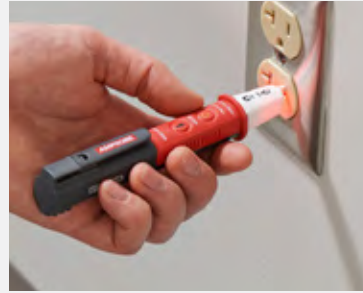
Test wall sockets for AC voltage
