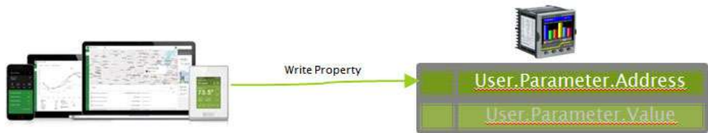
Figure 162 BMS Client writes address of required parameter
