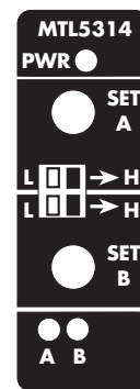
Figure 6.74: Top label, MTL5314, showing positions of trip switches and multiturn potentiometers
