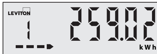
Figure 7 - LCD Appearance in Proper Operation (Example)
