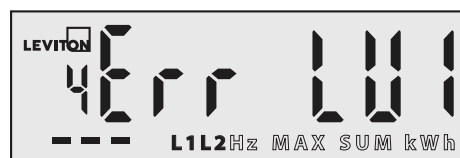
Error screen showing a low voltage installation error on Lines 1 and 2
