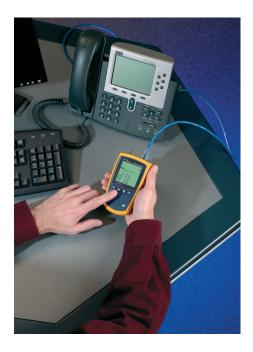
virtually any cable or wire pair, regardless of work environment. Use digital mode to locate high-grade data cabling (Cat 5e/6/6a) in bundles, or at switches, patch panels, or wall outlets. Or, use analog mode on voice-grade cabling (Cat 3 and below), as well as coax, security/alarm, and speaker wiring.
