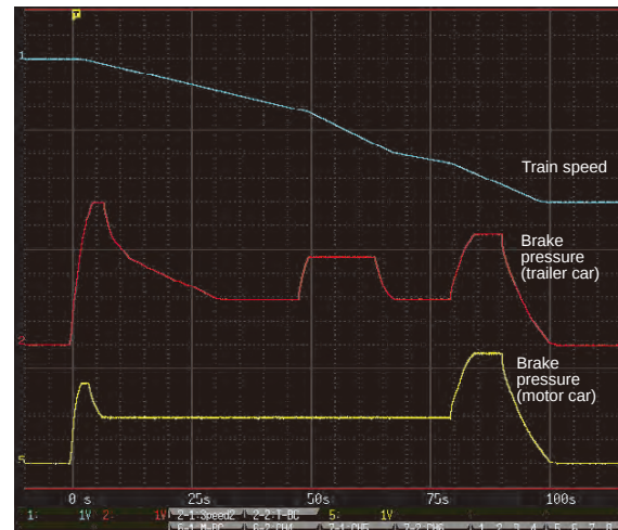
Appropriate brake pressure for the speed is analyzed with simultaneously recorded brake pressure and vehicle speed
