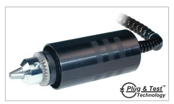
Series R50 smart sensors measure bi-directional torque for a wide variety of applications across virtually all industries. Contain a Jacobs chuck for up to 0.5 in [12.7 mm] diameter samples, bits, or fixtures. The sensors can be used as hand held devices, or mounted to a test stand. Capacities available from 10 ozFin to 100 lbFin [7 to 1150 Ncm]. Compatible with Mark-10 indicators (sold separately) through unique Plug & Test™ technology.
