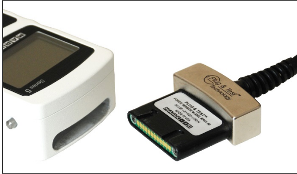
Fig. 3.1 Appropriate orientation of the Plug & Test® connector.
