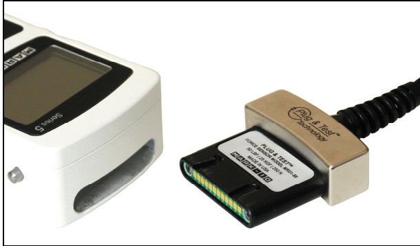
Fig. 3.1 Appropriate orientation of Plug & Test™ connector.
