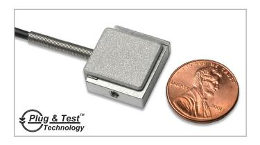
Series R04 smart sensors are designed for tension and compression measurement applications with tight space constraints. These extremely compact force sensors feature threaded holes on two sides, which can accept a variety of hooks and implements. Capacities available from 0.25 to 100 lbF [1 to 500 N]. Compatible with Mark-10 indicators (sold separately) through unique Plug & Test™ technology. Includes a certificate of calibration with data.
