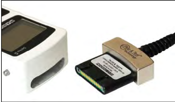
Fig. 3.1 Appropriate orientation of the Plug & Test™ connector.
