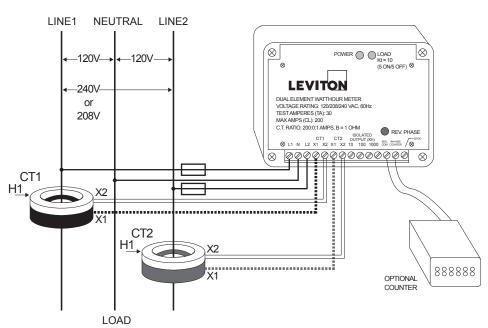
Leviton recommends solid core transformers (CTs) for revenue-grade accuracy. Our 100A and 200A color coded CTs assist with correct installation by indicating phase monitored. Split core CTs are also available upon request for applications where power cannot be interrupted during installation. Our 100-5,000 Amp Split Core CTs offer +/-1.0% accuracy.
