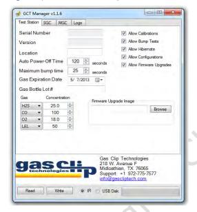
The GCT Manager software can communicate with the Clip Dock through IR or USB as selected by the radio buttons. IR communication is handled through Bay 1 of the Clip Dock and if the IR Link is placed into Bay 1. For IR communication, connect the Clip Dock to a charger and place the GCT IR Link into Bay 1. Direct USB operation with the memory stick connected to the PC offers faster transfers or configuration without a GCT IR Link.
