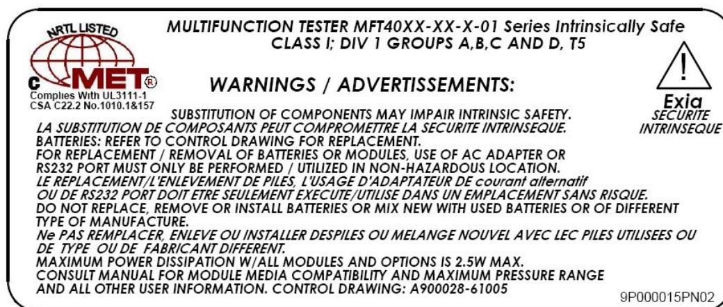
WARNING label for Intrinsically Safe MFT Units
