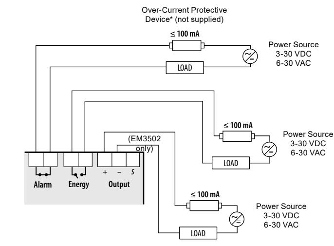
The solid state pulse outputs are rated for 30 VAC/DC nom. Maximum load current is 100 mA at 25°C. Derate 0.56 mA per °C above 25°C (e.g. 86 mA@50°C). \* The over-current protective device must be rated for the short circuit current at the connection point. \*\* All pulse outputs and communication circuits are only intended to be connected to non-hazardous circuits (SELV or Class 2). Do not connect to hazardous voltages.
