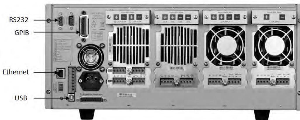
Figure 32 – Mainframe Rear Panel Communication Interfaces
