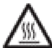
Caution, hot surface
