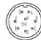
8-pin connector PC02E-12-8P Bendix
