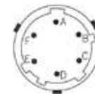
6-pin connector VPT07RA10-6PT2 (PT02A-10-6P)
