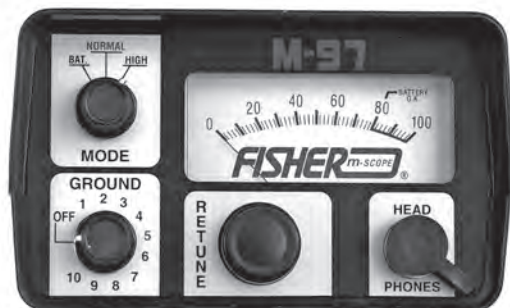
M-97 Control Panel
