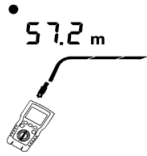
Figure 6.15 Open on Coaxial Cabling
