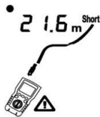
Figure 6.16 Short on Coaxial Cabling
