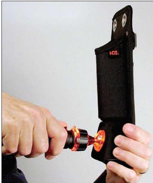
**WARNING:** This Detector does not detect DC. Flashing light indicates AC voltage. Do not use the LV-5 Detector or LV-PT Tester except as directed. Do not use the Tester with equipment other than the LV-5. Contacting voltage above 600V with the Detector or applying the Tester to energized circuits or equipment may lead to electric shock, severe injury or death. Refer all servicing to the factory.
