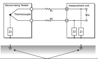
When using a thermocouple to measure temperature, noise can affect measurements unless both the device being tested and the measurement units are grounded. Although there is no problem if the measurement units is running on battery power, the instrument must be connected to ground if an AC adapter is being used.
