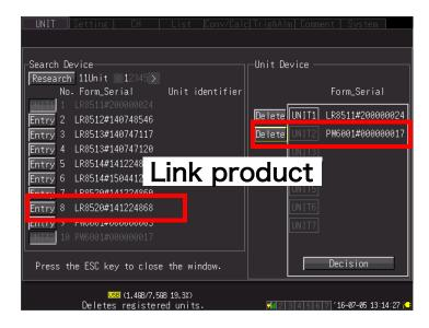
Product supporting LR8410 Link Model PW6001 (with the firmware version 2.0 or later installed)
