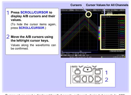
Cursor values can be displayed for all channels, or for only desired channels (p. 120).
