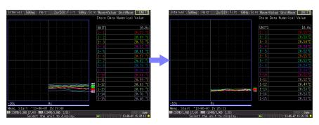
NOTE When scaling is automatically set by steps 1 to 6 on next page procedure, the measurement units are initially set to [V].
