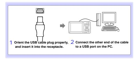
The first time the computer is connected to the instrument, follow the next steps to recognize the instrument.
