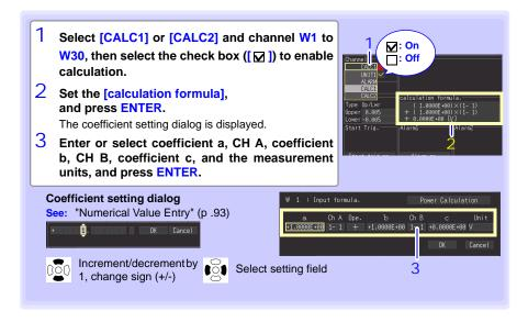
The calculation formula can be entered on the [Conv/Calc] screen. The calculation formula entered for channel W1 can be copied to other channels (p. 101).
