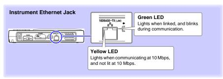
If the green LED does not light when connected to the LAN, the instrument NOTE or connected device may be damaged, or the cable may be faulty.
