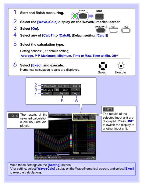
After measuring, calculation can be applied to a specified time span. Make any other calculation settings before specifying the calculation time span (P.188, 1
