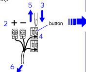
Push in the button on the Wireless Universal Unit's connector with a flatblade screwdriver.
