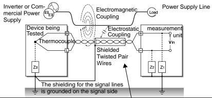
Keep the signal lines (of the thermocouple) away from wiring that is a noise source (such as power lines, etc.). It is also possible to shield the signal lines from electrostatic coupling and to block noise by grounding the shield.
