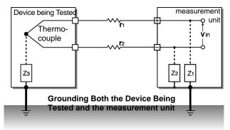
The wireless logger's design does not permit it to be grounded. If the unit is being affected by noise, operate it using battery power.
