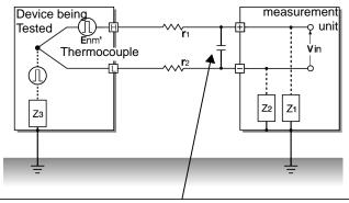
The capacitance of the capacitor should range from several µF to several thousand  $\mu F$ . Insert the capacitor between the "+" and "-" input terminals.
