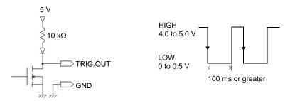
The signal is output even when triggering is not enabled. When triggering is NOTE not otherwise used, a trigger signal is output during measurement.
