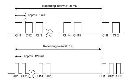
When the digital filter is off, the timing is the same as with a recording interval of 100 ms, regardless of the recording interval setting.
