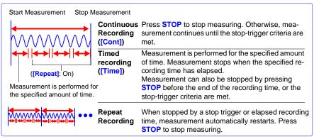
Measuring Method | Setting Method Continuous Sets the record time to [Cont]. Recording Timed recording Sets the record time to [Time]. This allows you to set the amount of time for which to record data. Repeat Recording Set [Repeat] to On.
