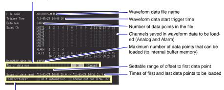
Unit registration information and communications settings (LAN, USB) can also be loaded. Select the checkbox for the settings you wish to load. Settings for unselected checkboxes will not be loaded.
