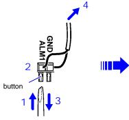
With the button held in, insert the cable into the cable connection hole.
