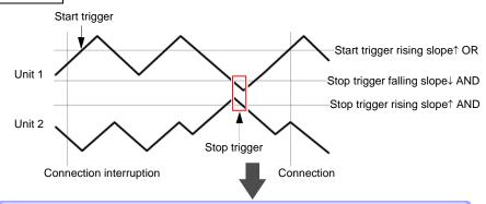
When unit 1 and then unit 2 are connected to the instrument (in that order)
