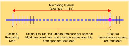
NOTE Statistical recording cannot be selected when the recording interval is set to one second.
