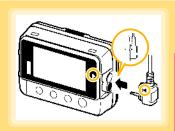
Align the triangle on the plug with the one in front of the sensor jacks, and insert the plug securely.
