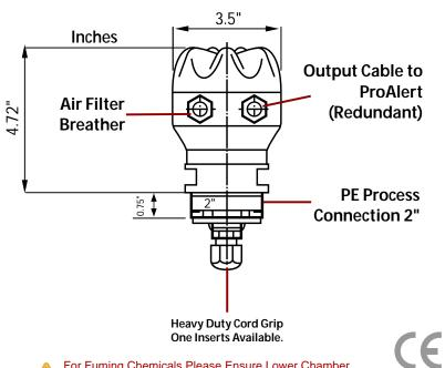
For Fuming Chemicals Please Ensure Lower Chamber is Sealed This will Prevent Internal Corrosion - RTV Silicone.
