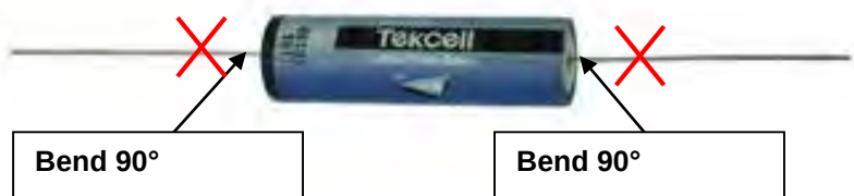
Figure 14: Shortening and bending the connections
