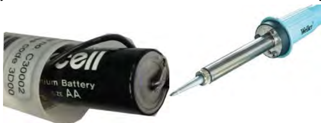
Figure 13: Unsoldering the battery
