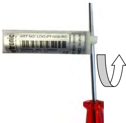
Figure 11: Unscrew cover with screwdriver
