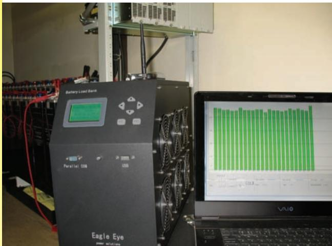
**DataView Software Allows The User To Monitor Discharge & Recharge!**
