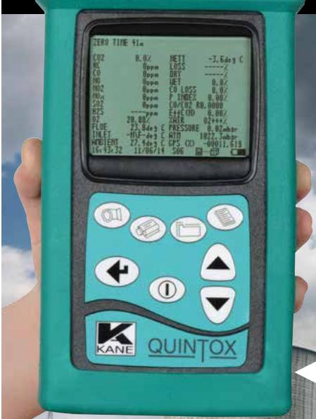
Independently tested by TÜV SUD to EN50379 the new **KANE9206 Quintox** is a cost effective & versatile emissions monitoring solution. Customised to your specific requirement the **KANE9206 Quintox** uses electro-chemical sensors to monitor Carbon Monoxide, Nitrogen Dioxide, Nitric Oxide, Sulphur Dioxide, Hydrogen Sulphide, and Oxygen. Combine up to five electro-chemical sensors with our infra-red measurement technology to monitor Carbon Monoxide (up to 10%), Carbon Dioxide & Hydrocarbons.
