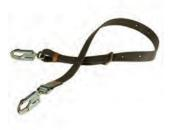
Klein's positioning straps work with Klein's climbing equipment for linemen. Made with exceptionally strong and long-lasting Klein-Kord, the straps are adjustable within a 2' range. Features a Gard snap hook with 5000 lb. (2268 kg) gate strength. The drop-forged, single tongue adjustment buckle has a corrosion-resistant finish. Depending on the application, choose a positioning strap that allows you to work at arm's length from the pole or other positioning anchorage.
