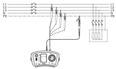
Fig.20 Example of Insulation resistance test on 4 wire-3 phase system.
