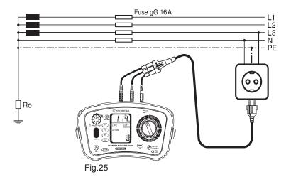
Max value of Zs for this example is 1.44  $\Omega$  (MCB 16A, characteristic C), the instrument reads 1.14  $\Omega$  (or 202 A on Fault current range) it means that the condition Zs x la  $\leq$  Uo is respected.
