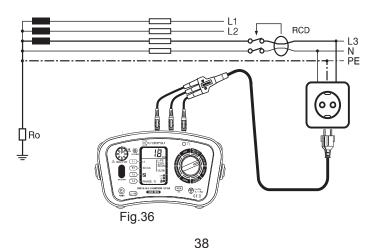
Practical example of RCD test with distribution leads.
