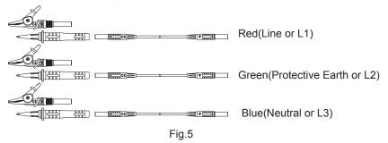
4. Earth Tests Lead(Model7228A) and Auxiliary Earth Spikes
