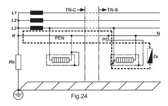
According to the International Standard IEC 60364, for TN system the characteristics of the protective device and the circuit impedance shall fulfill the following requirement:
