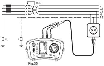
Practical example of single phase RCD test in a TN system.
