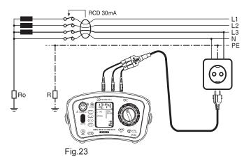
For this example the max permissible value is 1667  $\Omega$  (RCD =30mA and contact voltage limit of 50 V). The instruments reads 12.74  $\Omega$ , thus the condition RA  $\leq$  50/la is respected. However, considering that the RCD is essential for protection, it must be tested (Please refer to RCD TESTS section).
