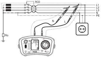
Fig.34 Connection for Line – Line measurement
