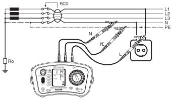
Fig.32 Connection for distribution
