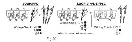
(3) Press the MODE switch(F1) and select L-N to measure Loop(L-N/L-L) or PSC or select L-PE to measure earth loop impedance or PFC. Display changes automatically as follows depending on the applied voltages while LOOP(L-N/L-L) or PSC is selected.
