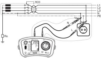
Fig.33 Connection for Line – Neutral measurement
