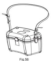
Pass the strap through the buckle, adjust the strap for length and secure.
