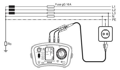
Fig.31 Connection for using Outlet
