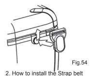
Match the hole of the Buckle and the protrusion at the side face of KEW6016, and slide it upwards.
