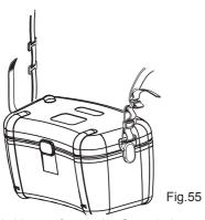
Pass the strap belt down through the buckle from the top, and up.
