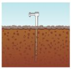
Earth measurements are possible up to 100kΩ\* of auxiliary earth spikes resistance.
