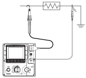
① Put the tip of the Line Probe (red) to the circuit under test. Then press the Test Button. The buzzer sounds intermittently during a measurement.
