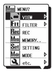
Move the cursor with the UP/DOWN Keys or Shuttle Switch, and confirm the selection with the ENTER Key. Pressing the ESC Key while the Menu is being displayed closes the Menu Window. Items displayed with " " mark are accompanied with submenus. Press the ENTER Key to access to the submenus.
