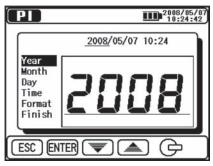
Select " @ " Clock Setting on the ENTER Menu (=>P.37). Adjust the time in a following order: [year], [month], [day], [hour], [minute] and [display format]. Pressing the ENTER Key confirms the entry and proceeds to next step. Press the ESC Key to return to the previous item.
