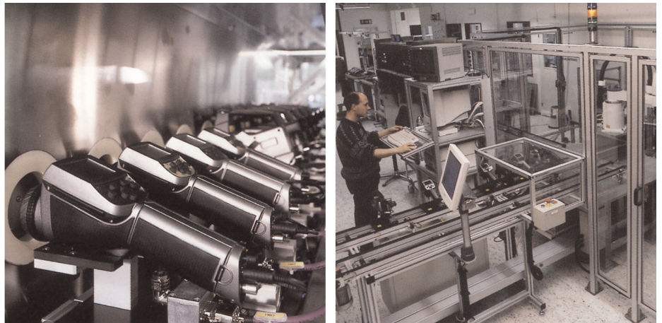
Figure 16.5 LEFT: Testing of infrared cameras in the climatic chamber; RIGHT: Robot used for camera testing and calibration
