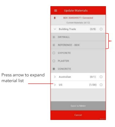
Greyed materials cannot be removed from meter (Drywall, Reference, and Douglas Fir)
