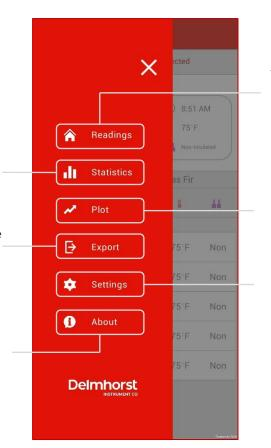
View the moisture content, time of export, material temperature, and pin type for each reading saved on the meter
