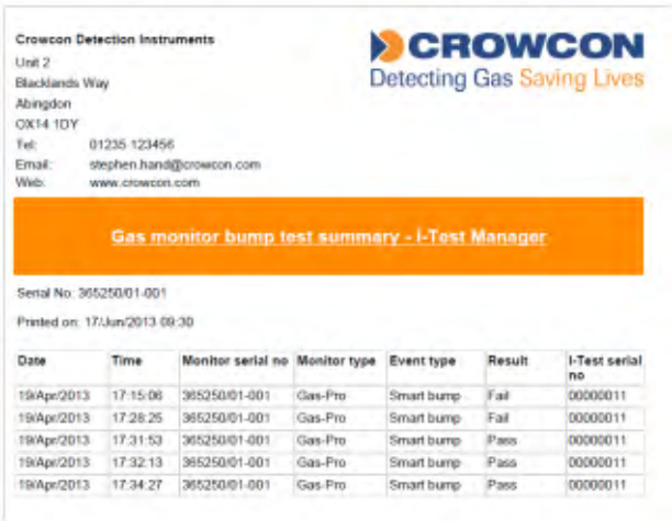
Figure 61: Gas monitor bump test summary report
