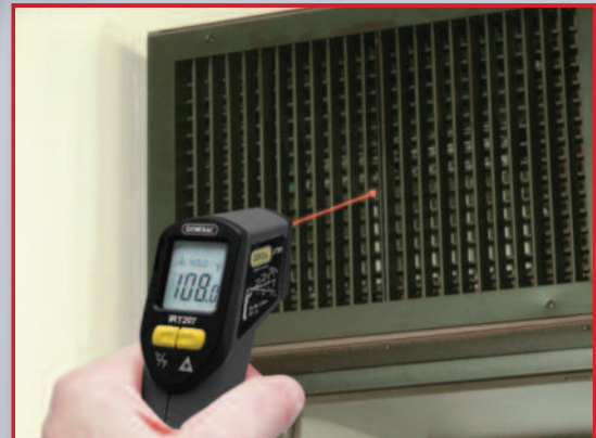
Performance-testing a new A/C system
