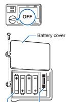
Batteries (LR6 ×4) Check the polarity.
