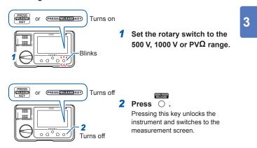
The screen is locked 1 minute after the last measurement or operation
