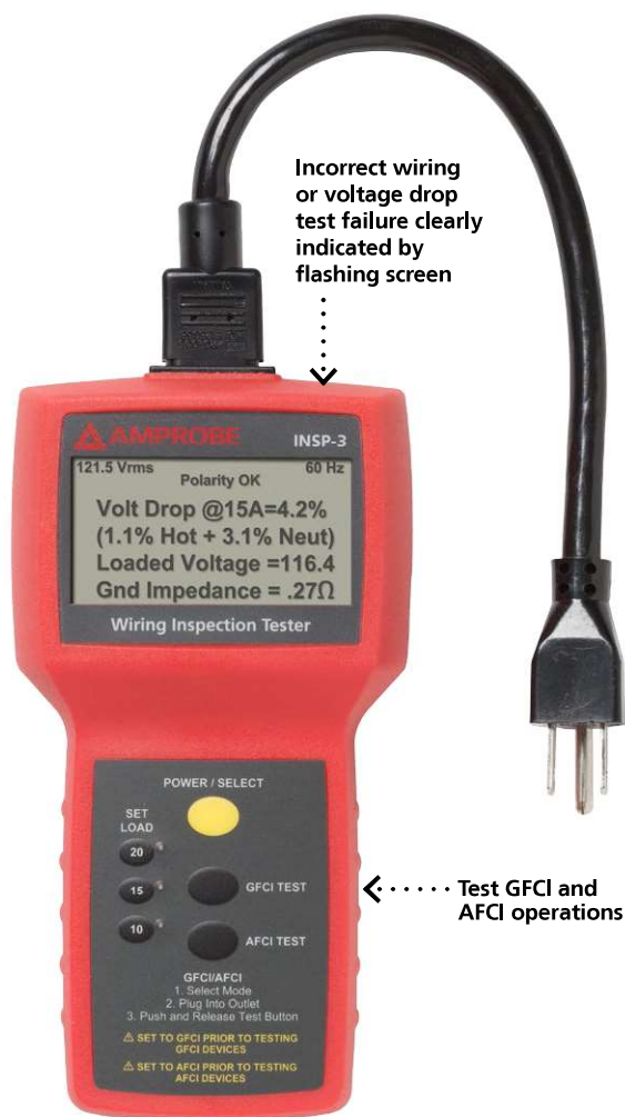
INSP-3 Wiring Inspector Tester
