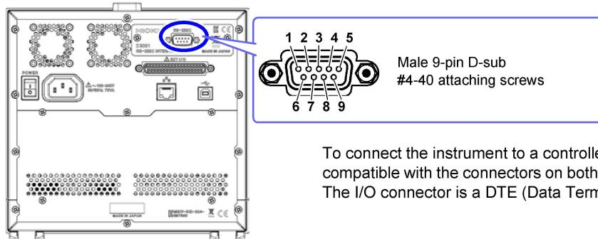
To connect the instrument to a controller (DTE), use a **crossover cable** compatible with the connectors on both the instrument and the controller. The I/O connector is a DTE (Data Terminal Equipment) configuration.
