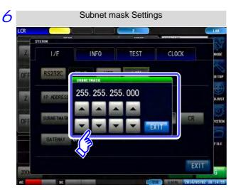
to set the subnet mask, to confirm the setting. and press **EXIT**
