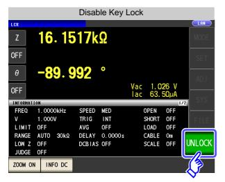
Press UNLOCK when the key-lock is enabled.
