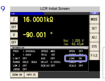
When the load compensation is valid for the set measurement conditions, ON appears on the LOAD parameter in the Initial Screen.
