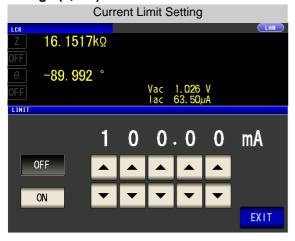
When the measurement signal level is a current (CC)
