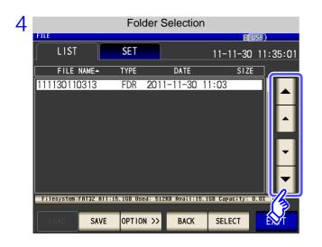
Using the ▲ and ▼ buttons, select the folder to which settings were saved with the all save function.
