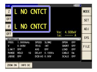
When an element other than a capacitor or a capacitor with a low DC resistance is measured
