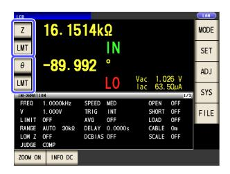
Judgment by comparator measurement and BIN measurement is performed for the first parameter and third parameter.
