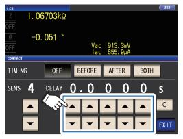
Settable range: 100 µs to 1 s Touching the C key causes the value to be set to 0 s.
