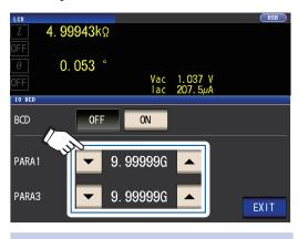
PARA1 Sets the decimal point position for the No. 1 parameter. PARA3 Sets the decimal point position for the No. 3 parameter.
