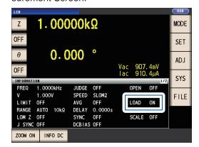
Use the same correction conditions for load correction as the measurement conditions when correction is performed. Use of different conditions will prevent load correction from being performed.
