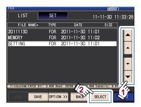
Select the setting file (SET) or panel file (PNL) to load with the ▲▼ keys and touch the LOAD key.
