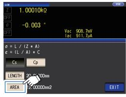
Enter the crosssectional area of the measurement sample and touch the **ENTER** key.
