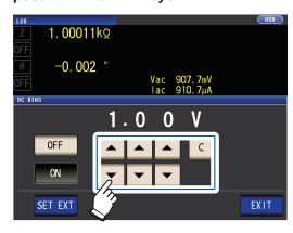
Settable range 0 V to 2.5 V If you make a mistake, touch the C key and reenter the value.
