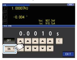
Use the ▲▼ key to change the trigger synchronous delay time.
