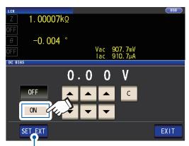
Touch this button when using an external DC bias unit (option).
