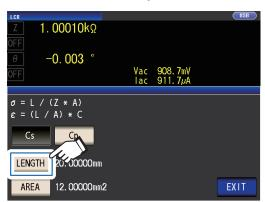
Enter the length of the measurement sample and touch the ENTER key.
