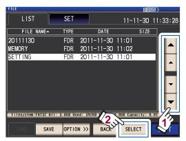
Using the ▲▼ keys, select the folder which settings were saved with the all save function and touch the SELECT key.
