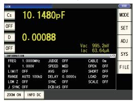
If OFF is selected in the parameter setting, a measurement value is not displayed.
