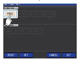
Enter the correction frequency with the numeric keypad, and touch the unit key to confirm the setting.
