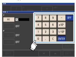
Settable range -999.999% to 999.999% When you do not want to set the upper and lower limit values, touch the **OFF** key.
