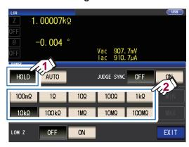
The measurement range is set based on the total impedance of the sample, measurement cable, and probe or test fixture.
