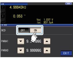
**OFF** Sets the output mode to judgment mode. (Judgment results will be output.) ON Sets the output mode to BCD mode. (Measured values will be output.)
