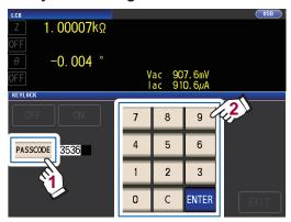
Use the numerical keypad to enter the passcode, and touch the ENTER key.
