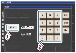
Settable range: 4 Hz to 8 MHz (default setting: 4 Hz)
