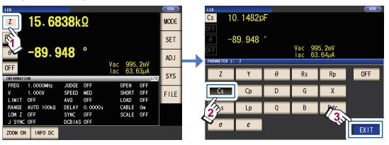
When you wish to perform DC in addition to AC measurement, set the parameter to Rdc.: "To perform DC measurement (DC resistance measurement)" (p. 40)
