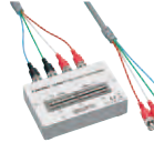
FOUR-TERMINAL PROBE 9140-10 Cable length 1 m (3.28 ft), DC to 200 kHz, impedance characteristics of 50 Ω, 4-terminal pair configuration, measurable conductor diameter: ø0.3 mm (0.01 in) to 5 mm (0.20 in)
