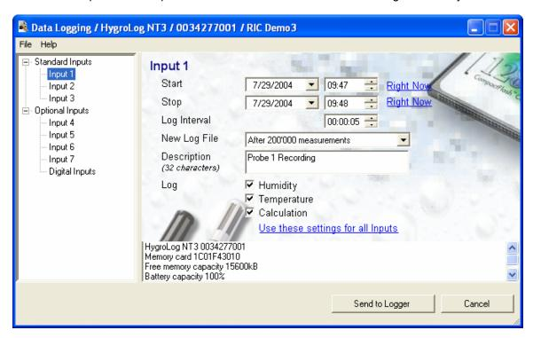
Both the standard and optional inputs are listed in tree located to the left of the dialog box. To select an input, click on it with the left mouse button.
