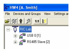
The instrument named RIC Demo1 has the RS address 01 and is connected to a USB port of the PC. The instrument named RIC Demo3 is connected by RS-485 to RIC Demo1 and has the RS address 02.
