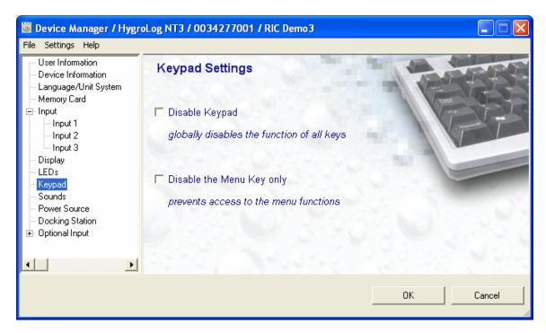
To prevent tampering with the logger or to prevent changes resulting from the accidental pressing of keys, the keypad can be completely disabled.
