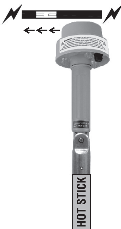
Fig. 2: Finding a cable fault
