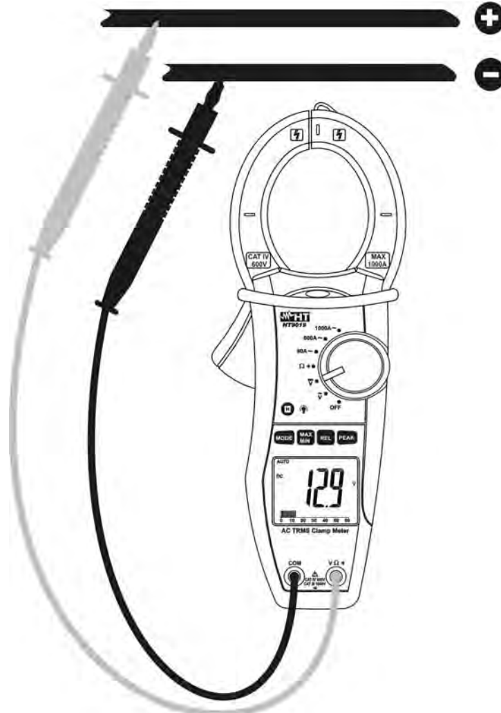
Fig. 4: Taking DC voltage measurements
