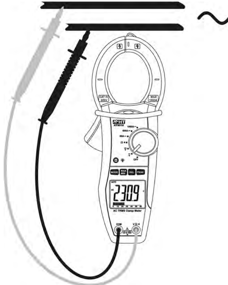
Fig. 3: Taking AC voltage measurements
