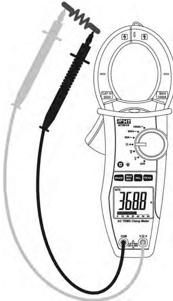
Fig. 5: Taking Resistance measurement and Continuity test
