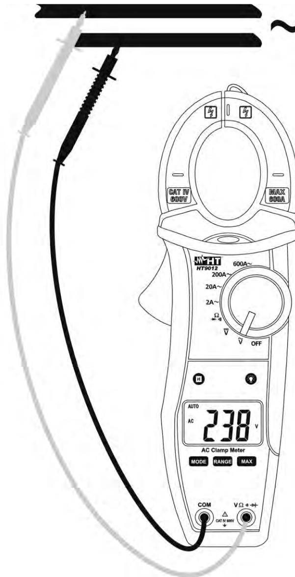
Fig. 4: Taking AC voltage measurement
